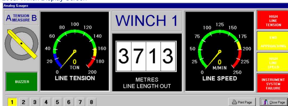
Local Winch Display Screen
